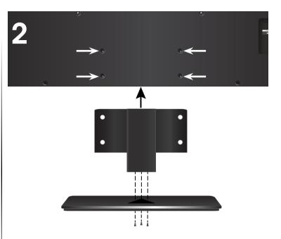
Align the base with the neck piece and tighten three (3) of the included Phillips screws with a Phillips screwdriver as shown.
